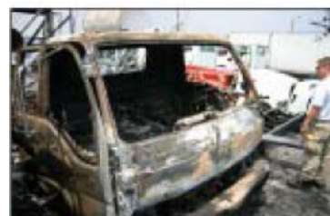
Another burned-out car 220 feet away due to rocketing cylinder fragment
