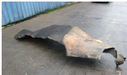
750-lb tank fragment landed near employees (both photos from CSB report)
